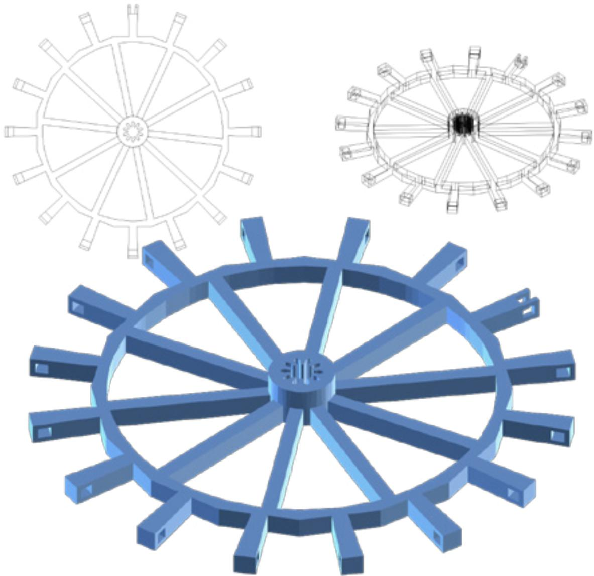
*Second omni wheel design in its simple polygon mesh form*
