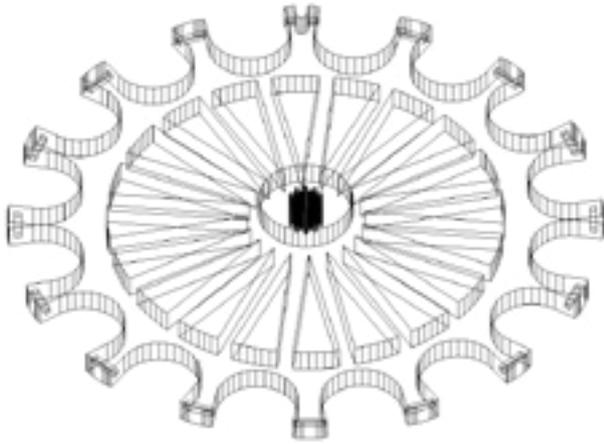
My first design was based on a simple wheel with spokes, holding 16 wooden balls in place with a wire.
