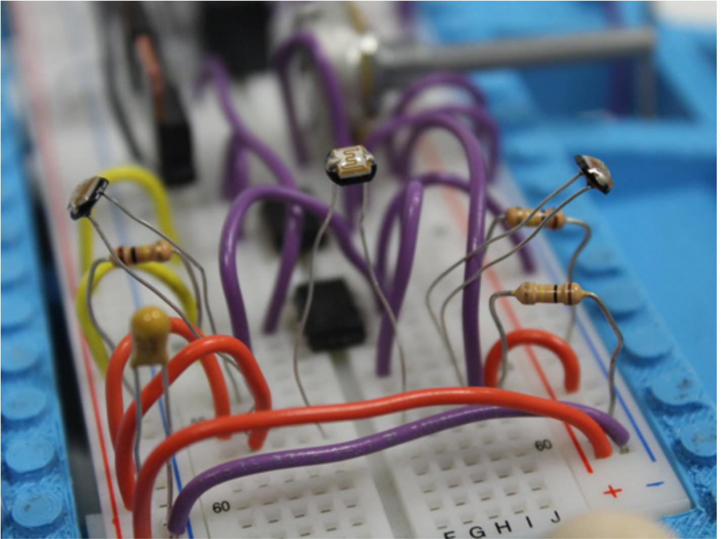
*Close-up of the photoresistors for triggering the motors (middle) and controlling directions*
