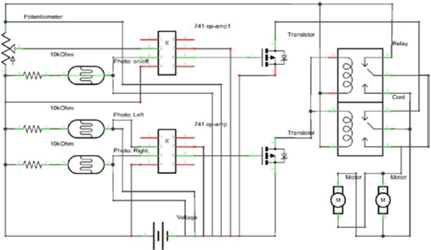
In my attempt to layout a first circuit, I divided the machine into two separately working modules. One part should control the X- and the other part the Y-axis of actions and reactions.
