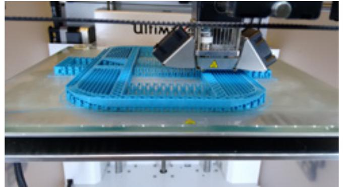
*Printing in process, starting upside down and building on support structure*
